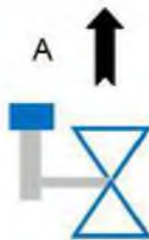
Counterweight mounted on the left (when looking in the flow direction) and dropping in anti-clockwise direction Counterweight mounted on the left (when looking in the flow direction) and dropping in clockwise direction
