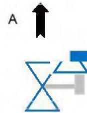
Counterweight mounted on the right (when looking in the flow direction) and dropping in anti-clockwise direction Counterweight mounted on the right (when looking in the flow direction) and dropping in clockwise direction
